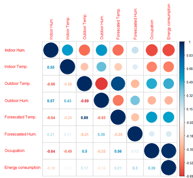
Figure 7. Cross correlation between influential variables in energy consumption. Done with a native routine in R: corplot.
